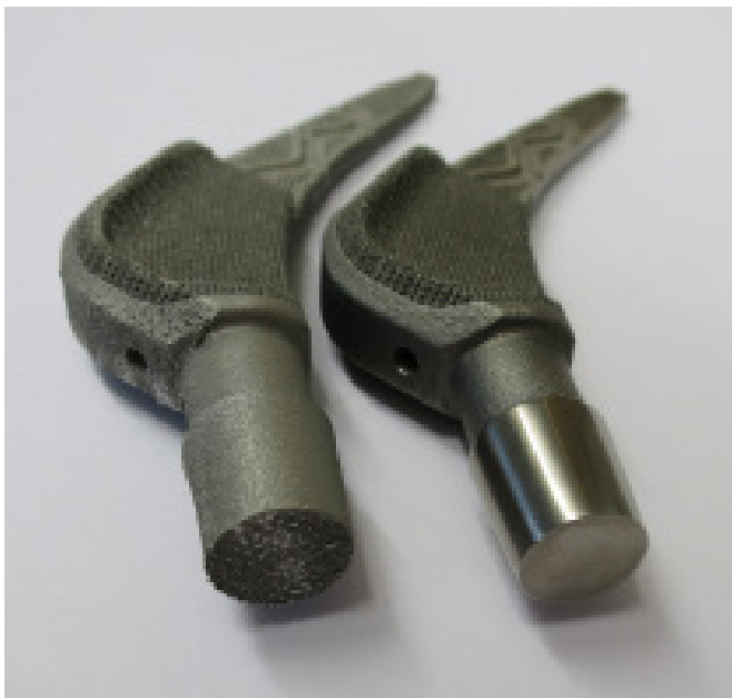
FIG. 5 MUGETO® femoral hip stem as built (left) and with polished functional surface (right) 7)
